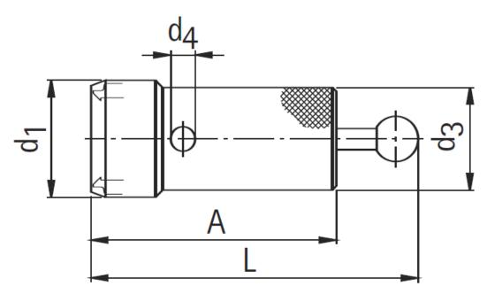
Used for installation and removal or dismantling KS clamping cartridges (standard and high pressure clamping cartridges). The assembly tool makes insertion and removal of the clamping grippers, even on multi-spindle heads, an easy operation.
