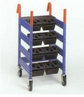
**Standard specifications:** 2 swivel casters (1 with brake), 2 fixed casters, 2 safety hand grips, 2 safety uprights, 4 aluminum profile rails, 1 deposit board with rigid rubberized surface, capacity 500 kg, weight 43.50 kg, color blue, LxWxH = 620x590x940 mm **Ref. No. 129.13**
