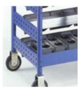
2 rectangular steel sections can be added lengthwise, accommodating 8 additional TUL tool carriers. This arrangement is well suited for long tools.
