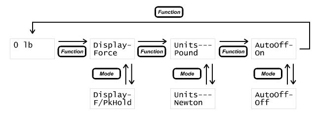
**Force:** displays only the force on the top line of the display.
