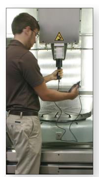
(rotating) conditions, verifying chuck holding force allows manufacturers to improve the repeatability of a manufacturing process by checking actual holding force – too much force can distort parts, while insufficient force can cause parts to come out during machining. In addition, regular verification of holding force is a critical preventive maintenance check.
