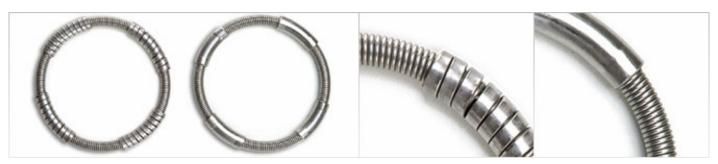
Roehrs automotive exhaust system springs are designed for use between the engine and exhaust system. They utilize a fully elastic suspension to minimize bending stress, and are designed for absorption of axial forces and torsion at temperatures up to 400 °C. The springs minimize noise and help to extend the lifetime of the exhaust system since they are constructed of corrosion resistant materials.
