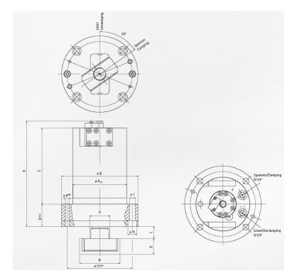
The hydraulic die clamping system with pull-back rotational style clamping is designed to clamp tools automatically at the press slide or on the table.
