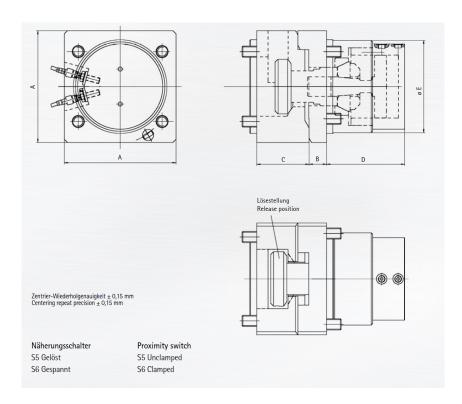
The hydromechanical self-locking gripper rail coupling is designed for automatic coupling of gripper rails on transfer presses. A vertical lift-out stroke is required for changing the tool. The coupling consists of a hard anodized aluminum housing, an axially movable tensioning rod and a hydromechanical self-locking clamping gearing. This configuration allows for high clamping forces and features a very high dynamic rigidity with minimum mass.
