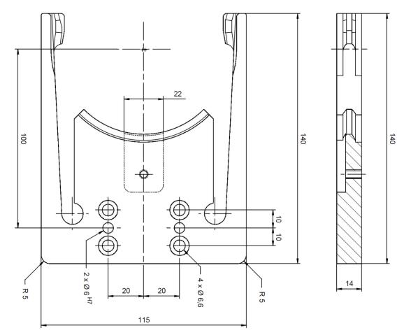
Standard duty spring steel grippers offer higher holding capacity and strength combined with a lower-cost design. Flexibility is maintained using a specialized spring steel and heat treat process. Grippers can be customized to meet specific mounting patterns. Contact us for taper sizes not shown.
