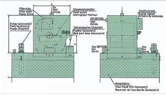
This type of filter can be used in all treatments where small chips and fine particles are to be filtered out of liquids even if these are of a rather high viscosity. This type of filter has proved its worth and efficiency not only in machining stations, but also in grinding machines. honing machines and wash water conditioning. This filter can be used as an individual system, but also for supplying several machines simultaneously.
