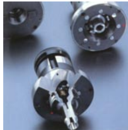
Adapter with clamping system for HSK.
