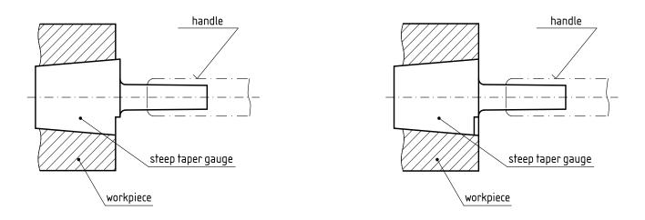
Insert taper gauge into the workpiece/spindle
